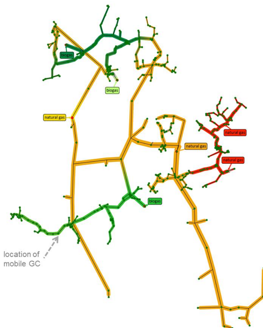
Figure 6: NGF grid with eight feed-in gases (natural gases: red, yellow, orange, biomethane: different green colors) and their distribution in the grid (monthly mean January 2017).
